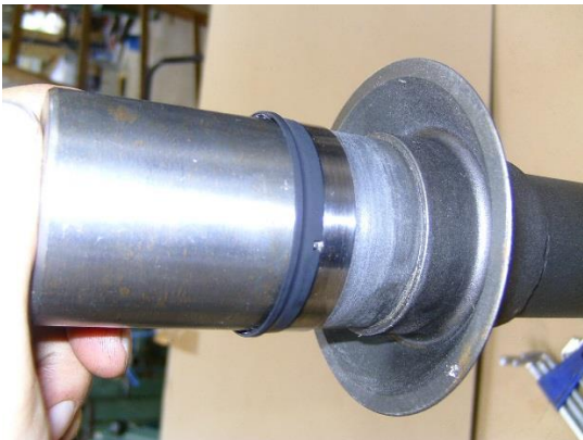
Seal pos 4.13 is replaced, important is positioning of this item
